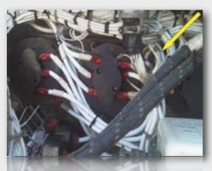
ensure everything was operational. The MIM calls for an electrical power test-set (AN/ ASM-439). This, however, requires a low-power turn, which wasn't feasible because 501 was in the hangar for a special inspection. Instead, the two AEs opted to manually energize the relay and check the connections. This procedure isn't in the manual, and therefore is not an authorized method of testing the relay.
